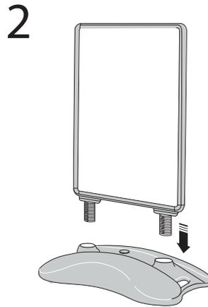
Insert the legs of the poster frame into the holes of the water-filled base
