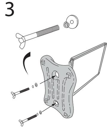
Rest the poster frame on its side, use the fixings shown to attach water-filled base to the poster frame
